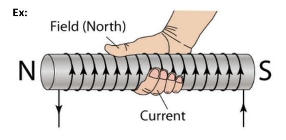
The current is represented by the black arrows. Wrap your fingers in the direction of the arrows, and you find that your thumb points to the left. That is the direction of the magnetic field.
