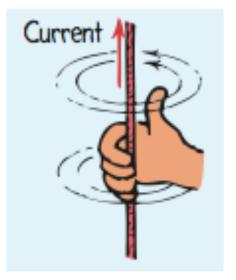
Your thumb follows the current, so you point your thumb up. The fingers on your right hand curl into the page on the right side of the wire and out of the page on the left side of the wire. This is the direction of the magnetic field.
