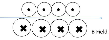
The magnetic field points INTO the page below the wire and OUT of the page above the wire.
