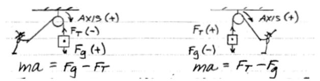
• These formulas apply regardless of the direction of motion. The force which tries to pull clockwise is (+). We do not assume to know which direction will dominate.
