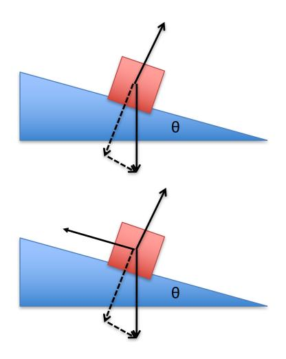
A 4 kg crate slides down an incline of 15<sup>0</sup>. The coefficient of friction between the crate and the incline is 0.45. What is the acceleration of the crate?
