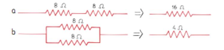
• Series  $R_{eq} = R_1 + R_2 + R_3 + \cdots$ • Parallel  $\frac{1}{R_{eq}} = \frac{1}{R_1} + \frac{1}{R_2} + \frac{1}{R_3} + \cdots$
