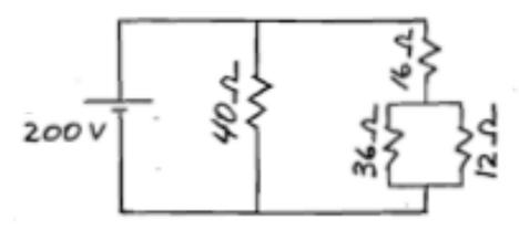
Find the voltage drop across each resistor, the current through each resistor, the total current supplied by the battery, and the total power delivered by the battery.
